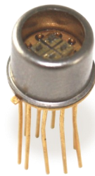
T0-5 Package—Up to 12 wavelengths
